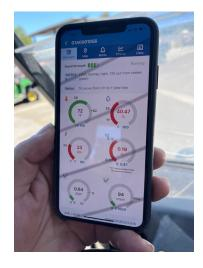
each sensor throughout the day. Thresholds were set for high and low soil moisture that would trigger an alert on the dashboard. Soil temperature and salinity measurements were also visible on the dashboard. The information was reviewed each day when programming irrigation run times.
